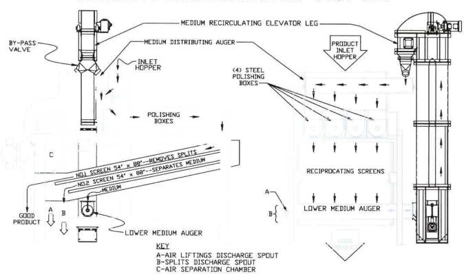
The "J" series is an extremely effective and unique polisher used primarily on edible beans and soybeans where a high degree of polish is desired. It is an inexpensive unit to operate and its gentle polishing action does not crack or split the product.
