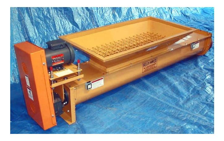
The vertical mixer spiral is force fed with a 9" screw feeder directly connected to the mixer downtube 6" above floor level. The 24" x 48" x 45 degree inlet hopper provides for convenient and metered loading of the mixer batch. The top of the hopper is located just 28" above floor level
