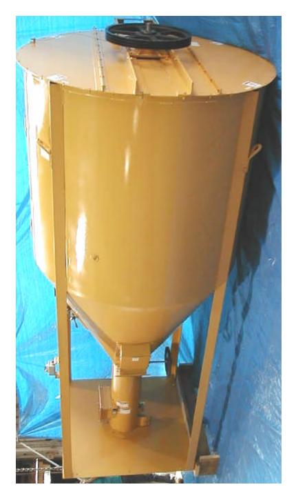
Overall view of vertical mixer illustrates 10" rack and pinion discharge gate and force feed inlet in down tube just 6" above the floorplate. V-belt drive is shown at the top.
