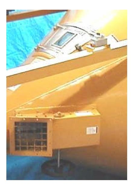
The maintenance panel in the mixer cone with a protective interlocking limit switch, the mixer discharge gate in the bottom of the cone and the installed Padlockable Protective Interlocking Electrical Control Switch are illustrated in these views of the vertical mixer.
