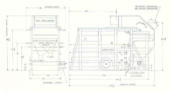
As is true with the Super 29-D the screens can be quickly set up as three tops and one finishing screen by re-arranging special catch-all spouts furnished.
